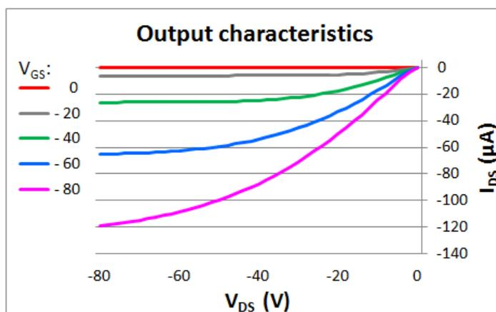
Figure 5: Typical output characteristic plot for the devices measured.
