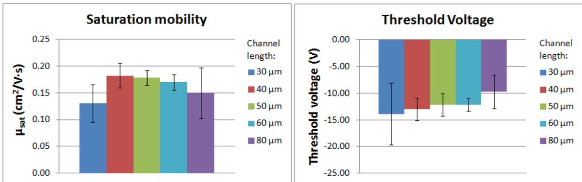
Figure 7: Data from all measured devices: the saturation mobility (left) and the threshold voltage (right). The error bars represent  $2 \times \sigma$ .
