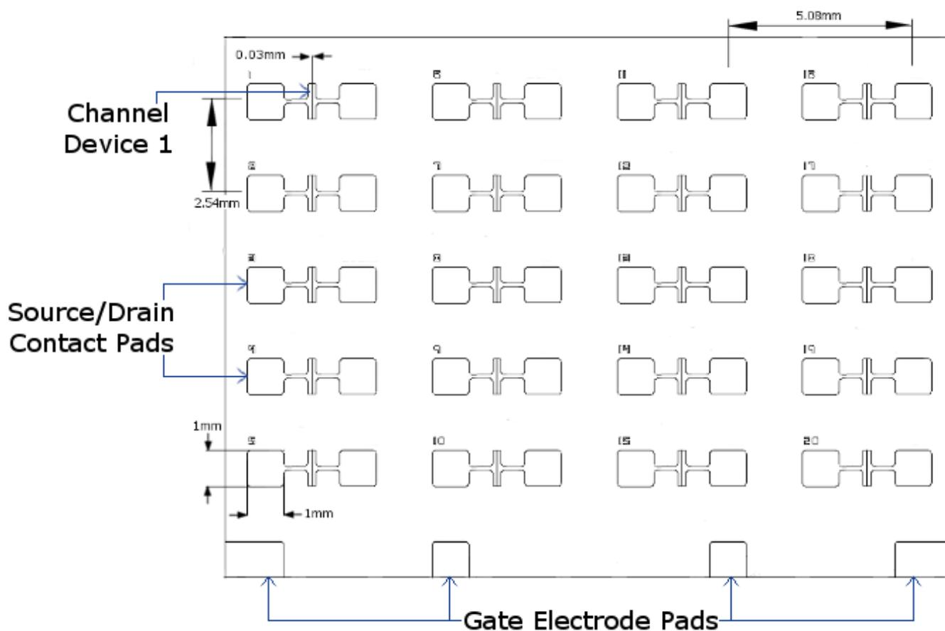
**Figure 1. Schematic of linear, high-density, constant-channel-length, pre-patterned silicon substrate for OFET fabrication.**
