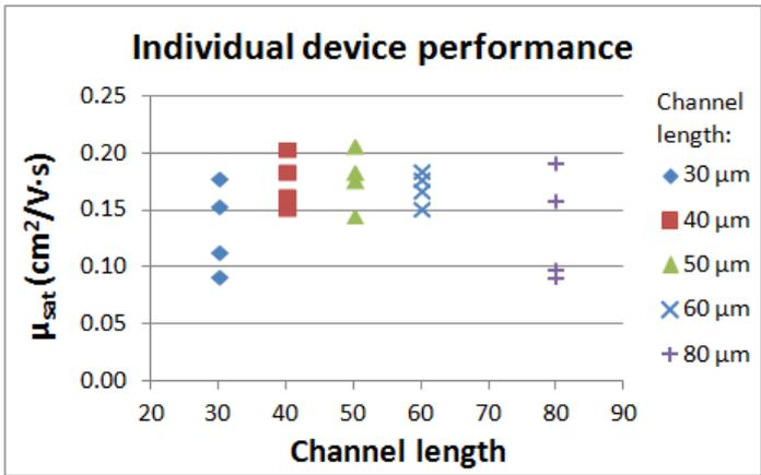
Figure 6: Saturation mobility of the 20 individual devices on the HD substrate.
