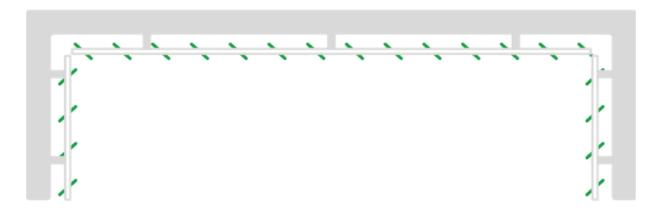
Your bracket will be 75mm which allows a clearance of approx. 25mm between the fabric and the facing surface.
