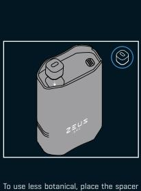
at the bottom of the heating chamber.
