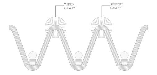
When determining placement for your fixture and electrical please note the wired canopy is on the left. The support canopy is on the right.
