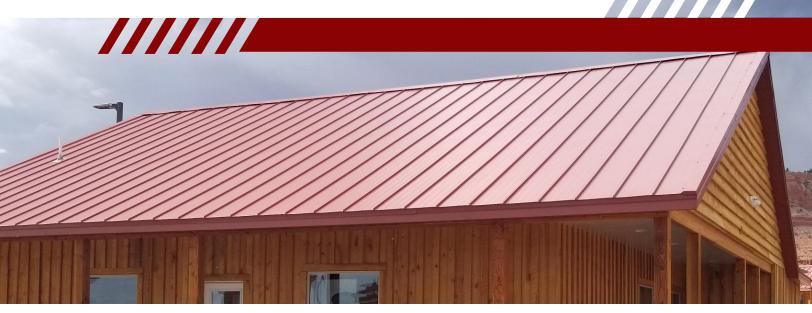
SL-16® is a sleek and rich looking, contemporary standing seam, hidden fastener panel system ideal for residential applications. SL-16® panels are formed from high tensile strength, using 29- and 26-gauge steel, which is protected with a Galvalume® coating. Our state of the art Signature® 200 paint system is then applied, providing years of warranted protection including Energy Star Compliance, Class A UL Fire Rated, and UL 2218 Class 4 rated for impact resistance.
