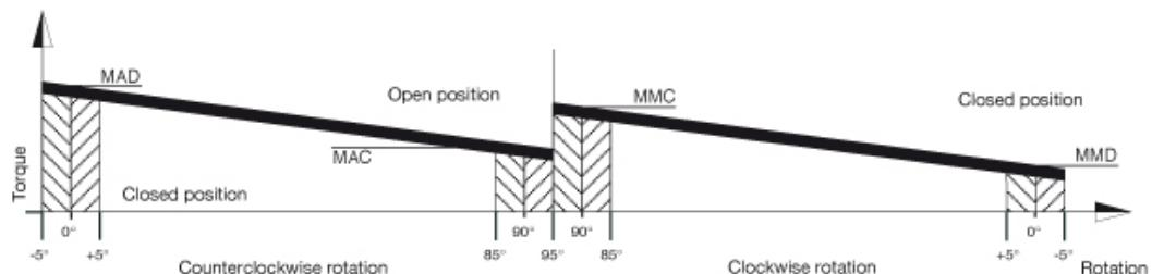
With reference to the above diagram the torque of a spring return actuator is not constant but decreasing. This is due to the action of the springs that when compressed during air actuation counteract the piston movement and accumulate energy which will be available in a decreasing way during the rotation inversion.
