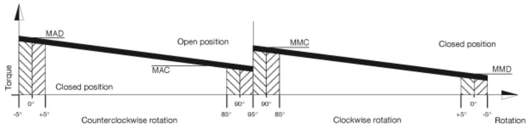
With reference to the above diagram the torque of a spring return actuator is not constant but decreasing. This is due to the action of the springs that when compressed during air actuation counteract the piston movement and accumulate energy which will be available in a decreasing way during the rotation inversion. The torque given by the actuator is defined by four fundamental values.
