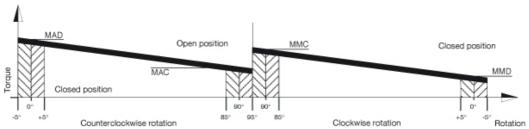
With reference to the above diagram the torque of a spring return actuator is not constant but decreasing. This is due to the action of the springs that when compressed during air actuation counteract the piston movement and accumulate energy which will be available in a decreasing way during the rotation inversion. The torque given by the actuator is defined by four fundamental values.
