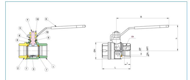
The Buna O-ring is fitted to the stem of the valve as the best possible protection against potential gas leakage under extreme duty, or low pressure applications. A secondary PTFE stem seal will also assure that the valve is suitable for use up to 366°
