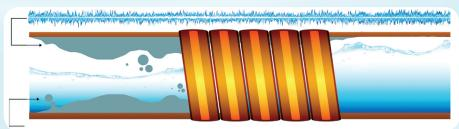
Electronic signal causes pieces of scale to begin to loosen, break off and flow out of pipe increasing water flow over time.
