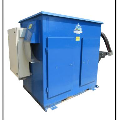
Flow can vary due to site conditions and altitude. Blower Performance is based on inlet air at standard temperature of 68°F and 36% relative humidity, and discharge at an ambient pressure of 14.7 psia. For performance at non-standard conditions, contact your authorized PRM representative.
