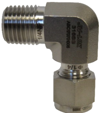
SS316CFEL90025TX025MTX 1/4" TUBE X 1/4" MNPT MALE 90° ELBOW
