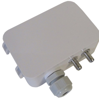
PGTLFMI005WCX 0-5"WC; 24VDC; 4~20 mA Output; 30 PSI Max.
