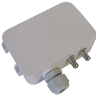
PGTLFMI040WCX 0-40"WC; 24VDC; 4~20 mA Output; 30 PSI Max.
