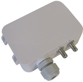
PGTLFMI001WCX 0-1"WC; 24VDC; 4~20 mA Output; 30 PSI Max.
