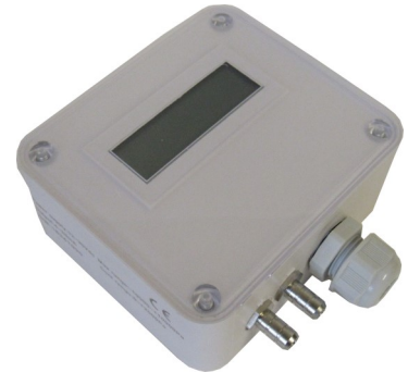
PGTLFMI010WCX With LCD Display 0-10"WC; 24VDC; 4~20 mA Output; 30 PSI Max.
