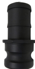
TYPE E MALE CAM LOCK/ HOSE SHANK 3/4", 1", 1-1/4", 2"
