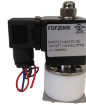
SV025DHFP2114NPT 1/4" PTFE Solenoid Valve 120V, PTFE Seal Direct Acting, Normally Closed
