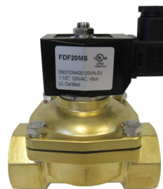
SV1502W21B120V 1-1/2" Brass NPT Port 120VAC, Viton Seal Normally Closed
