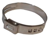
Single ear hose clamps or pinch clamps are easier to install than worm-drive clamps—crimp the pinch points with pinch-clamp pincers for a secure hold.
