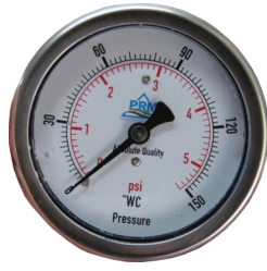
PGCNBTY630454B150WC 0-150"WC, 0-5 psi 2.5" Stainless Steel Case Back 1/4" Brass Connector
