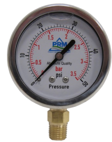
PGCNBTY630251850PSI 0-50 psi, 0-3.5 bar 2.5" Stainless Steel Case Bottom 1/4" Brass Connect
