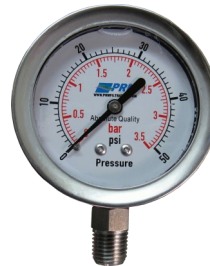
PGCNBTY63015350PSISS 0-50 psi, 0-3.5 bar 2.5" Stainless Steel Case Bottom 1/4" SS Connector
