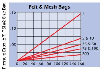
Flow GPM Water (1cps@70°F)
