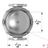
TYP 1 OF 4:  $\emptyset_2^1$ " FOOT HOLE 304 SS 40" 7 CARTRIDGE HOUSING
