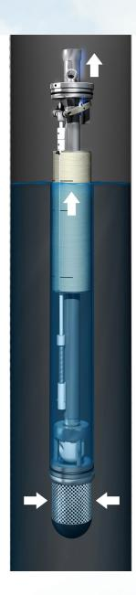
Fluid enters the bottom check valve and air in the pump exits the open exhaust valve.
