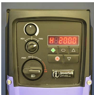
Fig. 8d Switch 3 set to 200 Hz
