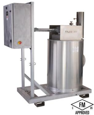
The FALCO 300 electric catalytic oxidizer treats air streams contaminated with volatile organic compounds. The catalyst provides VOC destruction efficiencies up to 99.5%. Operation, including startup, is fully automatic. Control system accurately regulates input loading and temperatures. The controls adjust a FALCO Vapor Control Valve (VCV) to maintain safe maximum input concentrations. Automatic shutdown results if temperatures exceed limits.
