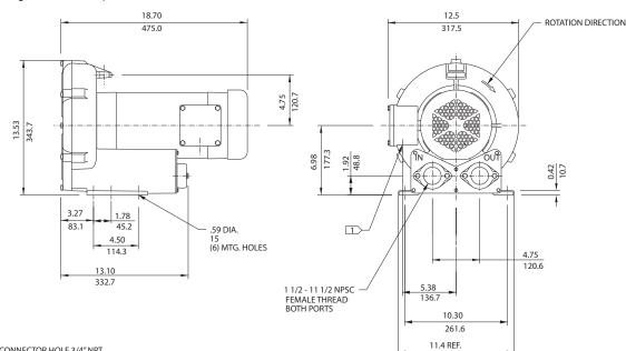
TERMINAL BOX CONNECTOR HOLE 3/4" NPT.
