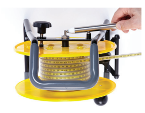
Figure 2 To Test the Entire System: Make sure sensitivity dial is turned fully clockwise. Touch the probe body to the standoff screw and probe tip to the stud (on axle) at the same time. The buzzer will sound if the system is okay.
