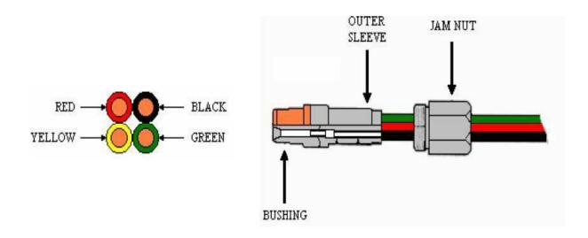
CONSTRUCTION: Jam nut/sleeve - 316 stainless steel, bushing - 4" Viton / 6" Polychloroprene
