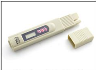
TDS meter. Fill lid with treated water & dip sensors in to check TDS. A 0 reading will mean a spot-free finish
