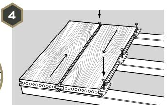
Take the next piece of deck and securely push into the Universal Clips. Now nip the screw to secure the Universal Clip against the board. **Do not over tighten**. Now repeat steps 3 and 4 to cover the deck, using one Universal Clip and screw on every joist. For a more natural finish, we recommend **alternating the direction of the wood grain** when installing the boards. If using the bullnose board, use this as your starting point.
