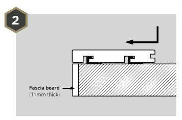
Insert the *HD Deck® Pro* bullnose deck board over the clips and push it forward. Secure in place with Universal Clips as required.
