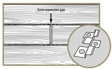
**SLIM CLIP ALTERNATIVE:** The Slim Clip can be used to close up the gaps between boards if preferred. Simply follow Steps 1-5, using the Slim Clip in place of the Universal Clip. **IMPORTANT:** the expansion gaps at the ends where the deck boards meet, must be maintained as explained in Step 5, .
