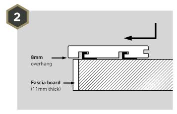
Insert the *HD Deck® Pro* bullnose deck board over the clips and push it forward. Secure in place with Universal Clips as required.
