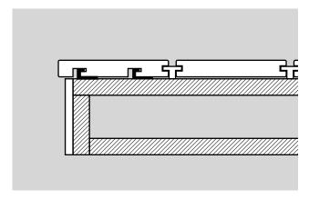
After installing the *HD Deck® Pro* bullnose deck board, as per the above instructions, use the Universal Clip to secure to the rest of the deck. See *Using the New Universal Clip* overleaf.
