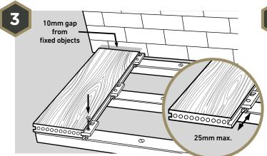
To secure the first board, use one Universal Clip and screw on every joist. Take a screw, place in the hole located in the Universal Clip and screw into the wooden joist. **Do not tighten at this stage.** Make sure the boards do not overhang the joist at the edge by **more than 25mm** and a **10mm expansion gap** should be left between the wall or other fixed objects surrounding the deck.
