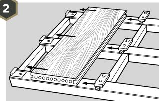
Place the first piece of decking on the timber frame with the decking running perpendicular to the joists. The first piece of deck may be secured with starter clips. **Do not screw or nail through** *HD Deck® Pro*, use one Universal Clip and screw on every joist.
