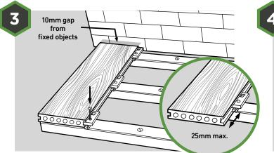
To secure the first board, use one Universal Clip and screw on every joist. Take a screw, place in the hole located in the Universal Clip and screw into the wooden joist. **Do not tighten at this stage.** Make sure the boards do not overhang the joist at the edge by **more than 25mm** and a **10mm expansion gap** should be left between the wall or other fixed objects surrounding the deck.
