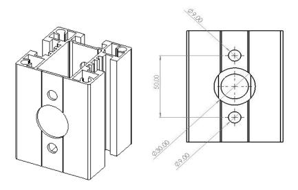
2. Now on the other side drill the holes shown below ensuring that the three centre holes line up with the holes at the front. Ensure that the Dia 3.5 holes go through 2 x wall sections to allow for the 32mm long self-tapping screws.
