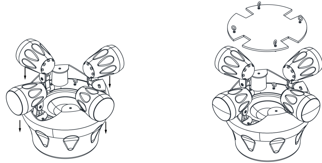
3. attach speaker to the subwoofer and repeat process for other 3 speakers.
