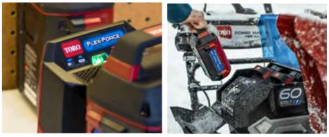
SAFE CHARGING The battery will only charge when it's at the right temperature. The easy to read on-board LED indicator shows when it's fully charged.
