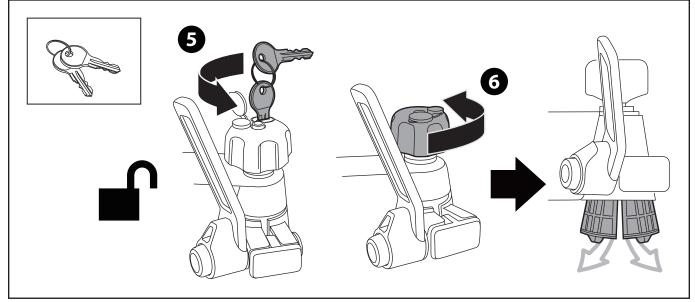
Caution: Compatible with 50mm towballs only. Do not fit to 1 7/8 towballs as this could result in damage to the rack.
