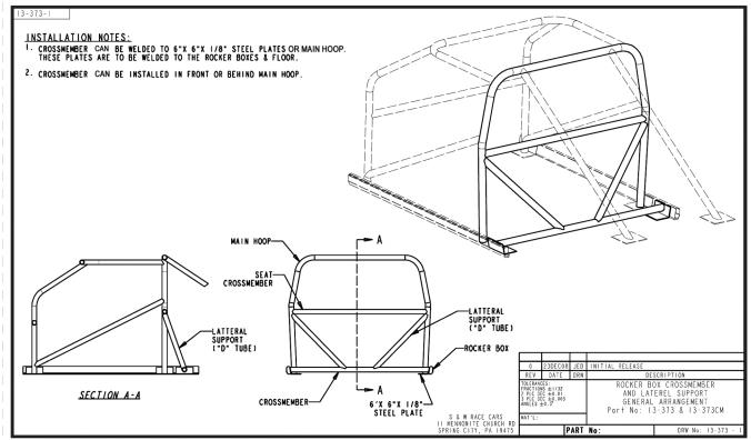
The drawing above shows the required method for installation of the lateral frame supports & crossmember now manditory on front wheel drive models
