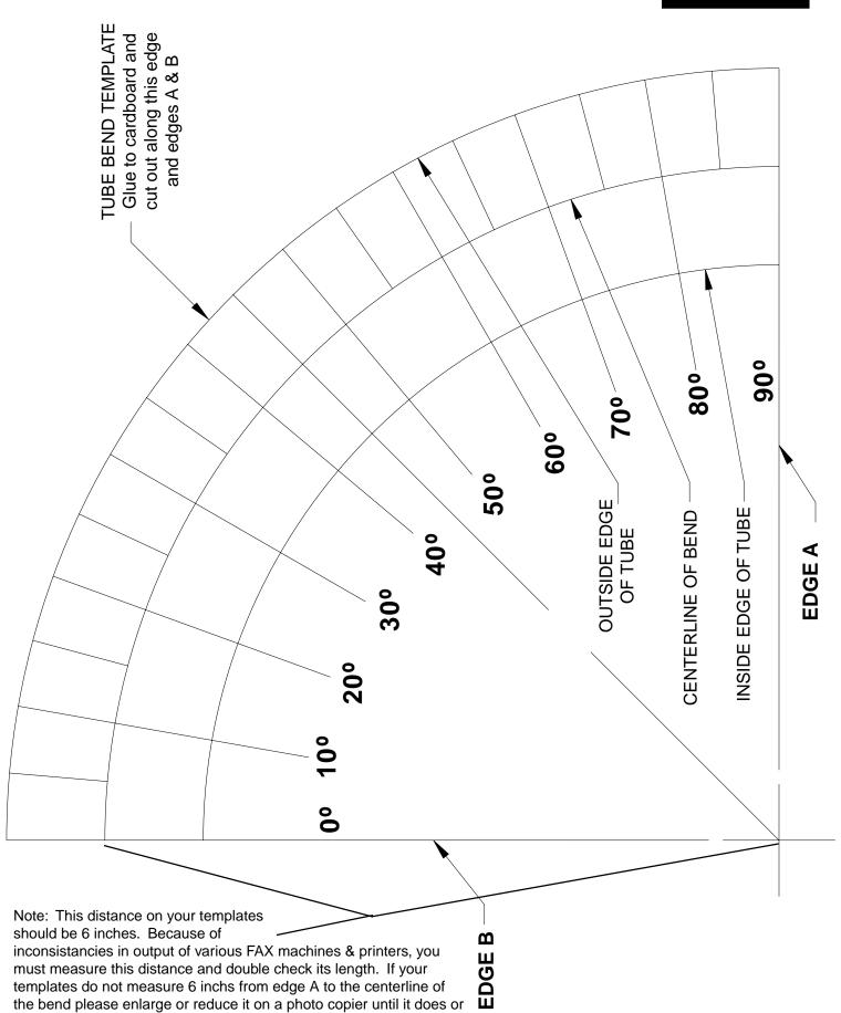
call S&W and we will send you the correct size templates. Failure to do this could result in an improperly bent roll bar.
