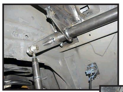
It has come to our attention that some 1993 - 2002 Camaros & Firebirds are equipped with an additional floor pan brace located near the top on the forward side of the rear housing area. Installation of part # 40-613 Torsional Anti Roll Bar on 1993 - 2002 Camaros & Firebirds equipped with this brace will require you to notch the brace for mounting bracket clearance. We suggest you bolt the right & left floor connecter to the torsion tube weldment and hold the assembly up in it's
