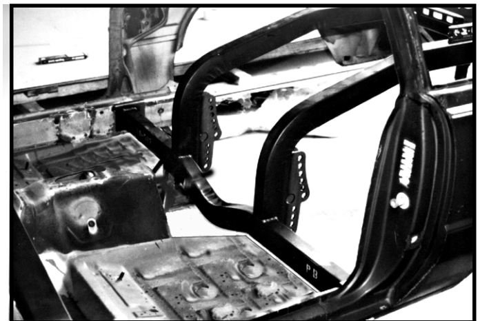
Photo #2 Transmission tunnel has been cut back farther than necessary for photo clarity. Your floor should be cut straight across.
