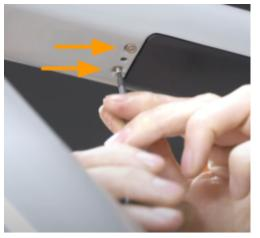
Next, unscrew the 2 **black** screws at the rear end of the Smartunit Main ECU. **!! Do not** remove the 2 other, silver-colored, screws next to it.
