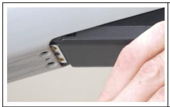
Great, now the Smartunit Main ECU can be placed back into the frame. Push the front end of the Smartunit Main ECU into the frame as shown in the picture.
