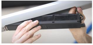
Now push the front end of the Smartunit Main ECU upwards and slide it into the frame, 1 cm beyond its mounting point.
