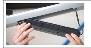
Now make sure the Smartunit Main ECU is pulled out, for **not more than 2-3 cm**, under an angle of 45°, so the connectors are partly visible as shown in the picture.
