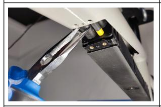
Use a pair of needle nose pliers to grab the motor cable connector and push it all the way back on the Smartunit Main ECU.
