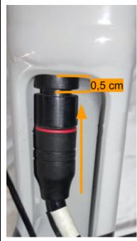
Keep the motor cable connector connected, and push the connector up into the front fork as shown in the picture.
