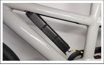
For the A5: you can gently lower the rear end of the Smartunit Main ECU up to the frame, as shown in the picture.
