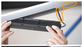
Then position the rear light connector into the backside of the frame while you push up the Smartunit Main ECU rear end.
