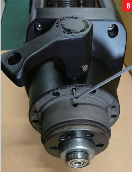
Once the L-handle is set to the desired orientation replace the two socket countersunk head screws securing the L-handle to the clutch mechanism using a 2.5mm Allen wrench to tighten.
