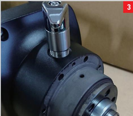
**3** Remove the T-handle from the gear housing.
