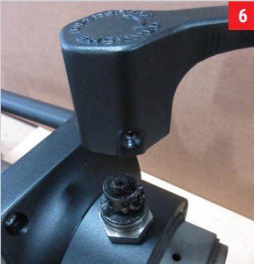
**6** Lift the L-handle from the clutch mechanism.
