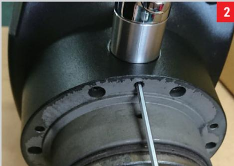
**2** Using a 3mm Allen wrench, loosen the M6 socket set screw securing the clutch T-handle threads in the gear housing.
