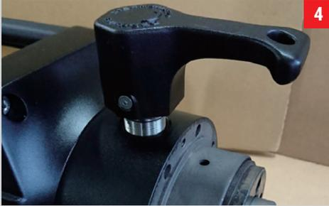
**4** Thread the L-handle (PN: 883236) into the gear housing making sure it is completely threaded into the housing. The final L-handle position could be adjusted in the following steps.
