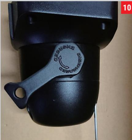
Reinstall the brake cover and secure using the four M5 socket head cap screws removed in step 1 using a 4mm Allen wrench.
