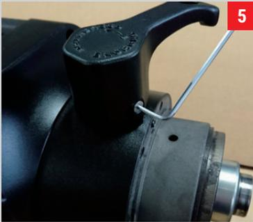
**5** Once the L-handle is threaded completely into the housing remove the two M4 socket countersunk head screws with a 2.5mm Allen wrench.
