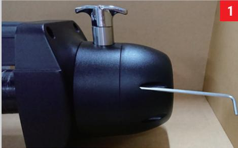
**1** Using a 4mm Allen wrench, remove the four M5 socket head cap screws holding the brake cover to the gear housing.
