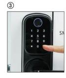
Press and hold the reset button for 5 seconds.
