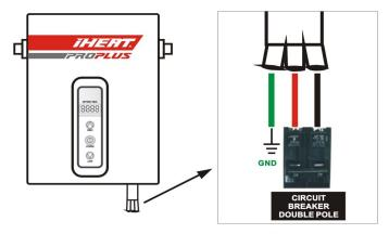
The electric heating elements operate at a constant temperature hot water at your chosen temperature setting. It is the rate of the water passing through the heater unit which determines the water temperature at any given setting. The slower the flow, less volume the hotter the water becomes, the faster the flow gallons per minute equals cooler water.
