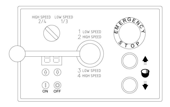
NOTE: TO START THE MOTOR, PRESS "ON" BUTTON, THE SPEED SELECTOR HANDLE MUST BE AT THE NUMBERS, INDICATING A SPEED, NOT AT AN INTERMEDIATE POSITION.
