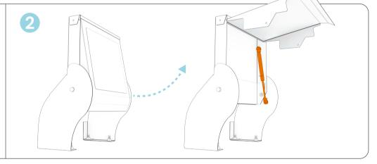
Use a small flathead screwdriver to **lift the clips on each end** of the gas spring, and pull the spring to remove.
