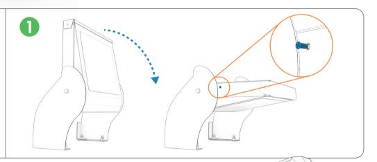
Place the step in a vertical position again and **lift the step cover** to access the **gas spring.**
