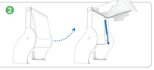
Use a small flathead screwdriver to **lift the clips on each end** of the gas spring, and pull the spring to remove.
