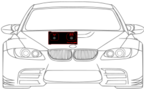
Front view of the vehicle. The rear part of the device, i.e., the power connector and GNSS antenna, should be visible
