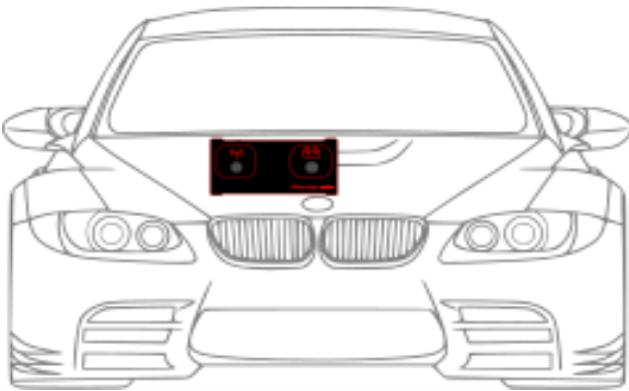
Front view of the vehicle. The back of the device should be visible, that is, the power and GNSS antenna connector
