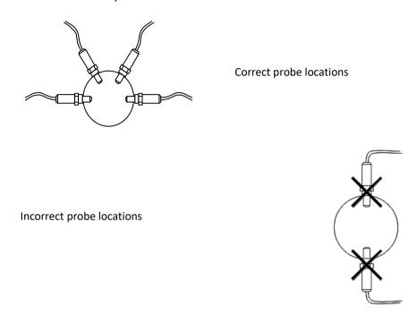
It is recommended that, if possible, the probe be placed in the exhaust pipe at least 1 m from the exhaust valves, to avoid excessive temperature, and 1 m from the end of the exhaust pipe, to avoid contamination with atmospheric oxygen. This is not mandatory and if necessary, can be located closer to the engine on short exhaust systems.
