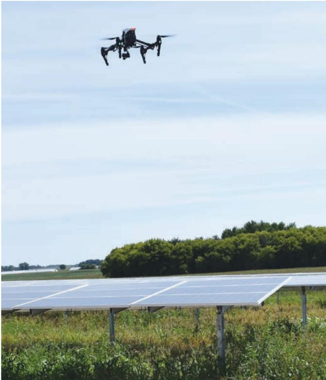
**Flight planning** Drone operators can tune the resolution of thermal scans by varying flight altitude. While high-altitude flights result in a faster survey, low-altitude flights provide more detail regarding defects.
