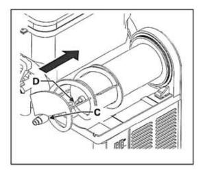
J. Set the bowl back in place; slightly raise head (C) of the auger so that it meets the seat (E) provided in the bowl and click into place
