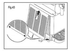
C. Using a dry brush or thick towel brush off any dust or dirt accumulated in the fins; then replace metal panel
