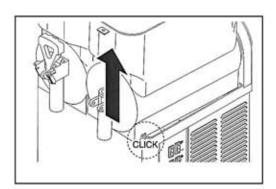
E. Remove the auger by pulling straight out, and remove seals (A & B)
