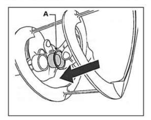
H. Lube seal (B) using provided food grade lubricant and reattach to machine
