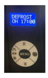
The Defrost settings help you to set your machine on a repetitive schedule, by creating a window of time you would like the machine to freeze / refrigerate on a loop.
