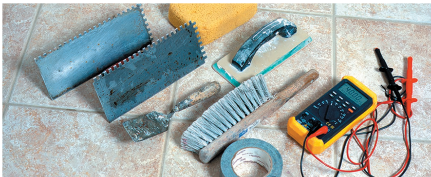
FIGURE 1.21: Assemble required tools
